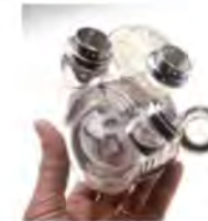
FIGURE 15: Biventricular electrically operated pusher plate design for a blood pump with four valves similar to that of the natural heart.
