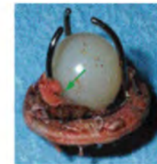
FIGURE 5: Thrombus formation at the seat of a ball valve as a result of the closing force of the ball against its seat.
