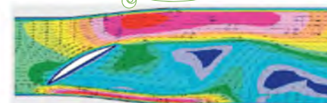
FIGURE 7: Flow patterns around a tilting disk valve generated by computational methods. Note the reversal of the velocity vector behind the tilted disk and the higher velocities at the periphery.
